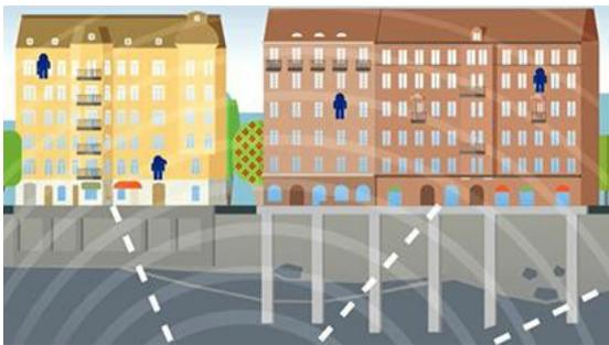
Vibrations in ground due to nearby blasting in rock
