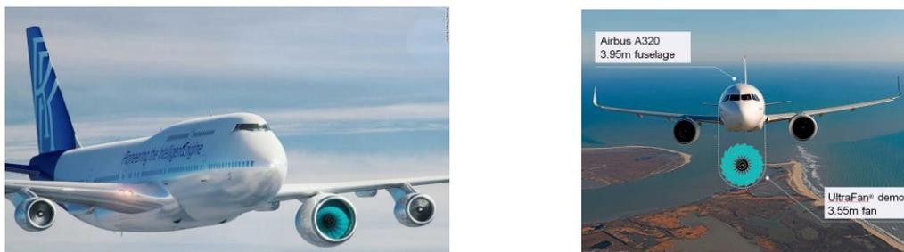
Figure 1: (a) Three engines installed on an aircraft. The middle one is an UHBPR engine (termed UltraFan) produced by Rolls-Royce and the others are normal engines. (b) Comparison of the diameters between UltraFan and the Airbus A320 fuselage.
