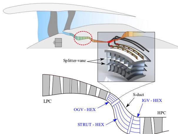
Figure 1: Concept of vane integrated HEX.
