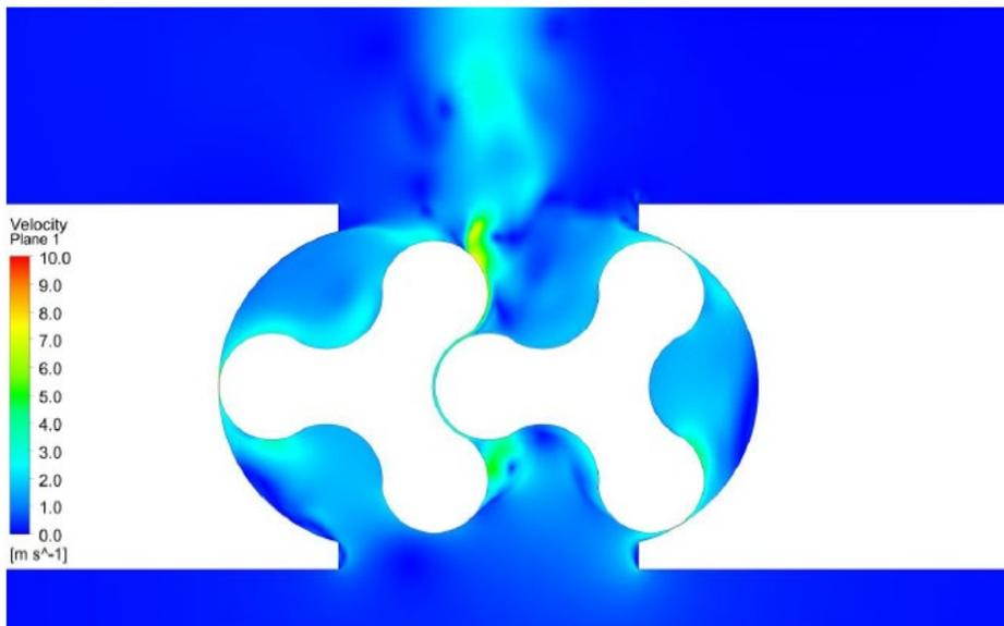
**2D CFD simulations of flow in a positive displacement pump from an ALPHEUS partner report.**
