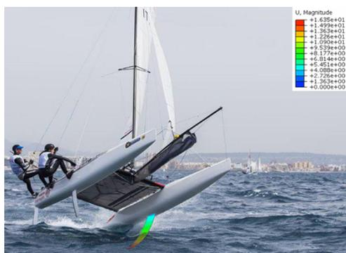
Figure 1: Hydrofoil subject to an extreme sailing load.
