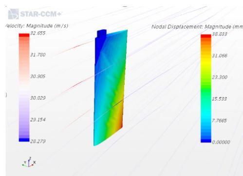
Figure 2: Aerofoil subject to wind tunnel loading and its ultimate deformation.
