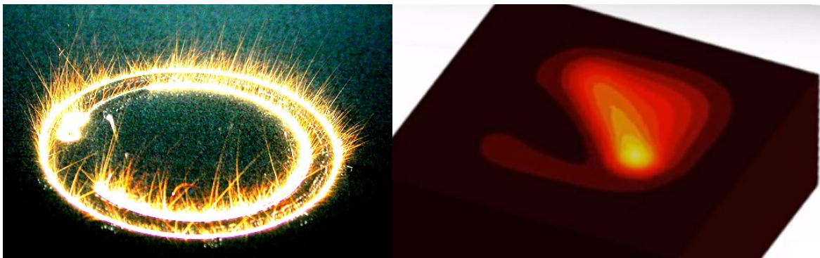
Figure 1 Left: Picture of Laser scanning. Right: temperature response from a meso scale model.
