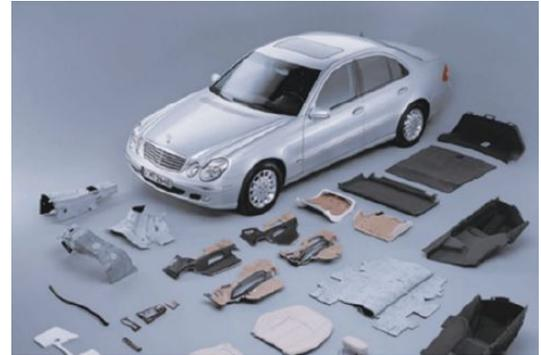
**Figure:** Components of an automobile made from biocomposites [Holbery and Houston (2006), JOM, 58 (11): 80-86]
