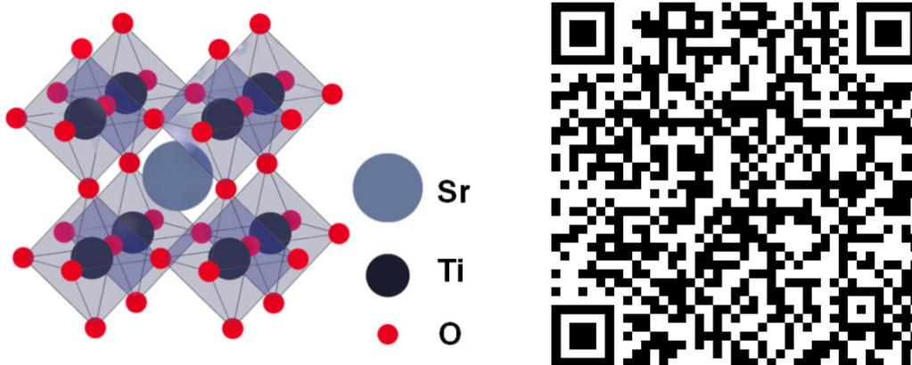
Left: Sketch of the strontium titanate crystal structure. Depending on the temperature, the precise ordering of the atoms will change, which in turn will affect how electrons move in the lattice. Right: The QR code links to a [popular blog entry](#) on the subject by thiscondensedlife.com called “Strontium Titanate – A Historical Tour”.
