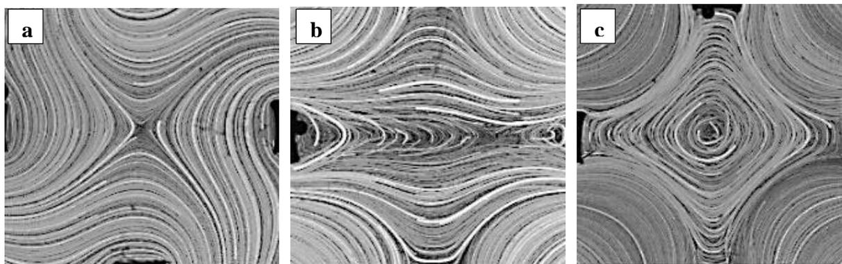
Figure 1. Streaklines for extensional (a), shear (b) and rotational (c) flows [1].
