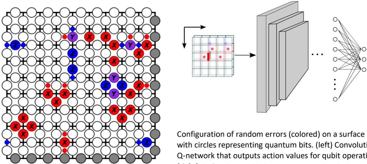
Configuration of random errors (colored) on a surface code with circles representing quantum bits. (left) Convolutional Q-network that outputs action values for qubit operations. (right) Code at <https://github.com/mats-granath/toric-RL-decoder>
