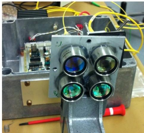
Figure 3: LIDAR sensor for ice detection
