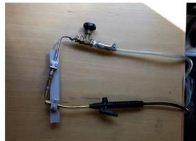
Device for manufacturing of glaze ice using separate nozzles for water and air. Glaze ice sample.
