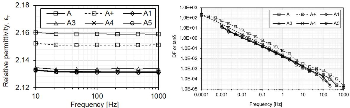
Figure 2 Relative permittivity (left) and dielectric loss factor,  $\tan\delta$  (right) of lubricant samples shown at 50 °C. Adding particles to the samples and electrically aging samples does not alter the relative permittivity and DC conductivity of the samples. The dielectric loss factor in Samples A1, A3, A4 and A5 is only slightly lower than that of Sample A.
