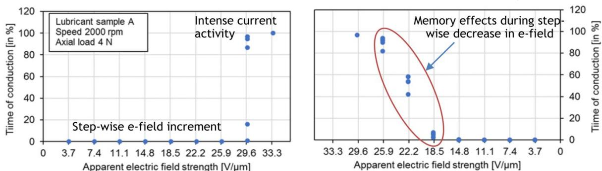
Figure 1 Breakdown of electrical insulation of bearing occurs at e-field of 29.6 V/μm, seen when e- field is step-wise increased. Upon decreasing the e-field after intense current activity, the bearing shows memory effects, where it fails to recover electrical insulating ability at lower values of e-fields.
