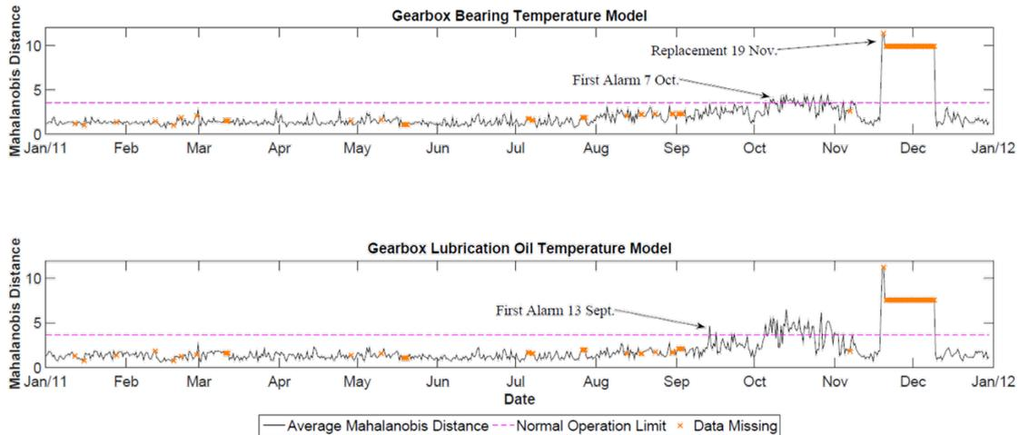
**Figure 1 Output from the ANN-based condition monitoring system for a wind turbine with gearbox bearing fault**
