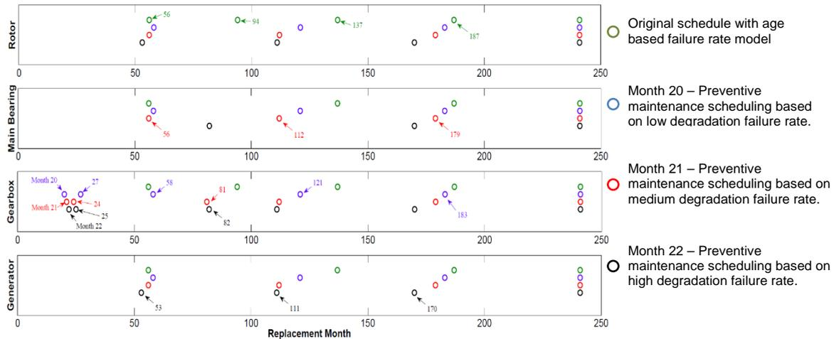
**Figure 3 A typical output of an optimized maintenance schedule based on condition based failure rate model for a test wind turbine**
