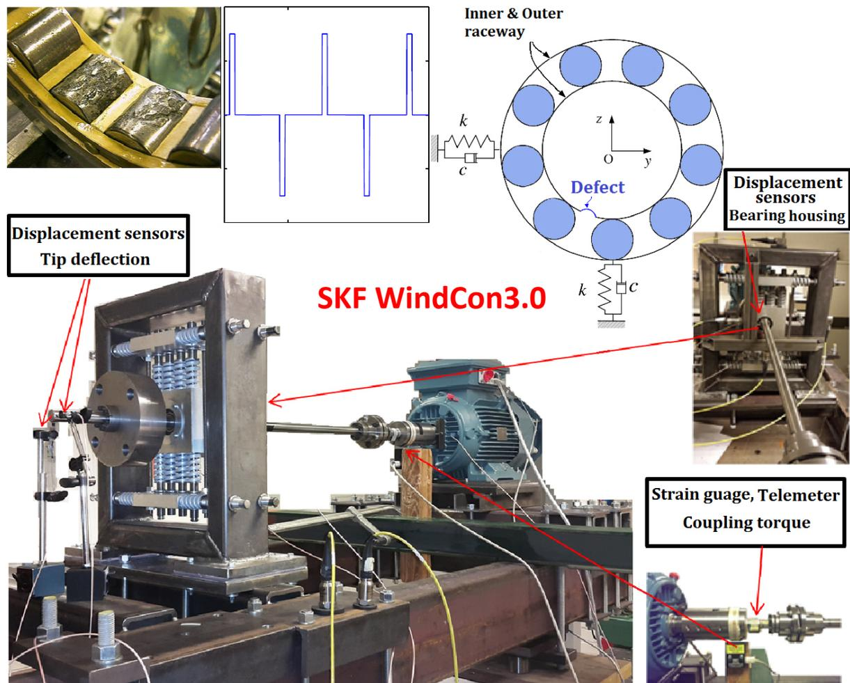
Fig. 1 The test rig of high speed subsystem of a drive train of a wind turbine
