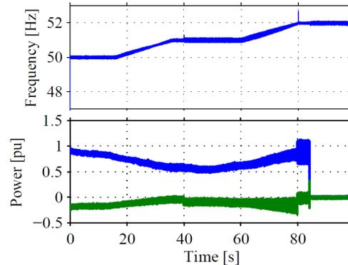
Fig. 4: Frequency variation test consisting of two consecutive frequency swells of 1 Hz (top), and active (blue) and reactive (red) power out of the wind turbine (bottom).
