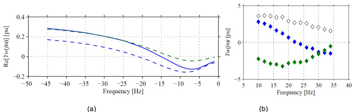
Fig. 2: Wind turbine admittance: Plot (a): real part of the admittance given by analytical model (dashed) and simulation model (solid). Plot (b): measured at Big Glenn by HVDC (blue: real part, green: imaginary part, and white: magnitude of the admittance).
