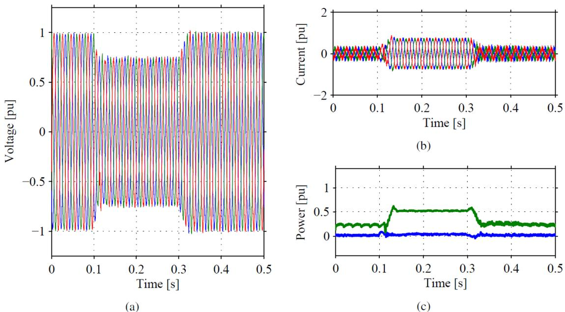
Fig. 3: Wind turbine under voltage dip test at low power production. Plot (a): three-phase voltage; Plot (b): three-phase current; Plot (c): active (blue) and reactive (green) power.
