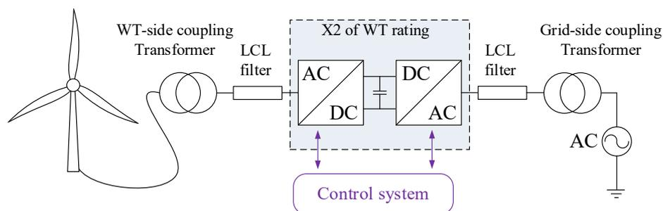
Fig. 1: Wind turbine connected to a Back-to-back VSC –based testing equipment.
