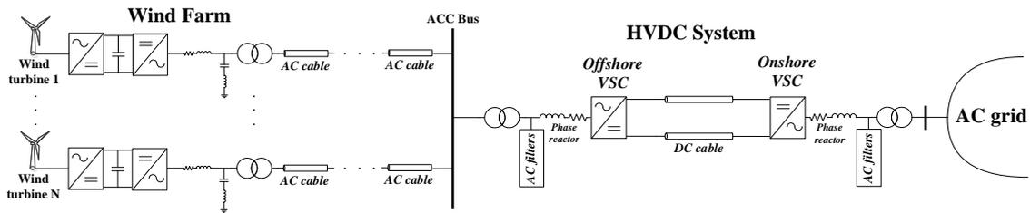
Fig. 1. Schematic of the offshore wind farm connected to the onshore grid through HVDC system.
