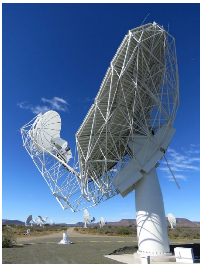
MeerKAT antenna with receiver containing LNAs from LNF. Courtesy of Onsala Space Observatory.
