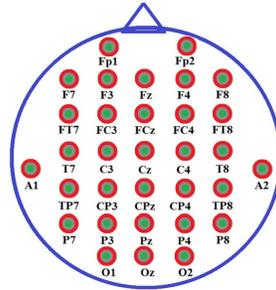
**Fig. 2.** The positioning of an EEG headset with 32 electrodes with their names as per 10-20 system standards.
