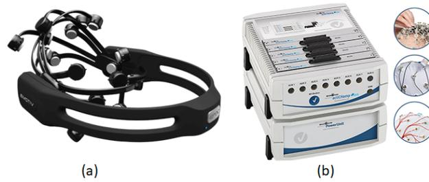
**Fig. 1.** EEG headsets: (a) Eemotive Epoc+ (14 electrode) [2] (b) ActiCHamp Plus (32-160 electrode).
