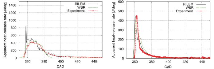
Figure 2: Apparent heat release rate for RILEM compared to the WSR model and experimental data for the full load case (left) and the part load case (right)
