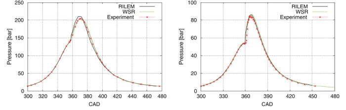
Figure 1: Cylinder pressure for RILEM compared to the WSR model and experimental data for the full load case (left) and the part load case (right)
