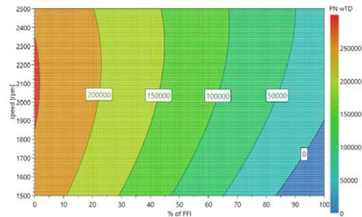
Figure 1. Solid PN measured with thermodenuder. Engine load of 7 bar IMEP, engine speeds ranging from 1500 to 2500 rpm and fuel injection mode changing from 0 to 100% PFI, R2 = 0.79
