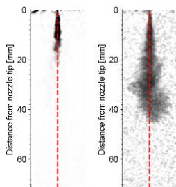
Figure 1. Visible and UV shadow images showing the extent of liquid and liquid+vapor phase fuel distributions.
