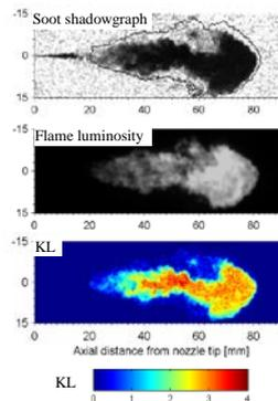
Figure 2. Soot shadow and luminescence images and derived KL factor in reacting Diesel spray.
