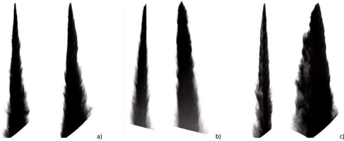
Figure 2: Spray visualization matching the in-nozzle flow depicted in Figure 1: centrally arranged 90° orifice (a), centrally arranged 75° orifice (b) and eccentrically arranged 90° orifice (c). The left image shows the spray formation from the sharp edge nozzle and the right image from the hydro-erosive ground nozzle configuration. The lower part of the sprays is cut-off due to the optical limitations of the spray chamber.
