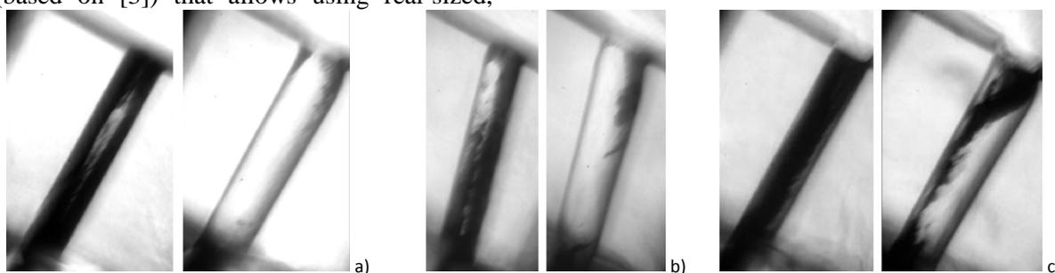
Figure 1: In-nozzle flow visualization for three different nozzle designs: centrally arranged 90° orifice (a), centrally arranged 75° orifice (b) and eccentrically arranged 90° orifice (c). The left image shows the sharp edge and the right image shows the hydro-erosive ground configuration. Dark areas indicate cavitation.
