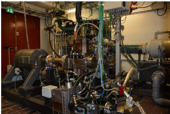
**Figure 1: Experimental setup of the heavy-duty Diesel engine coupled to the WHR system.**
