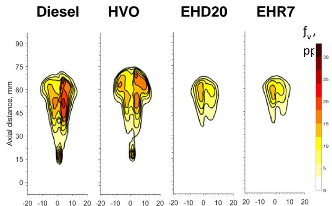
Figure 1: Soot volume fraction, ppm at combusting condition (550°C, 4.6 MPa,  $p_{inj} = 120$  MPa), 1.5 ms ASOI.
