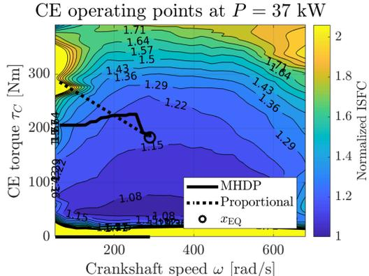
Figure 1: Representative combustion engine (CE) transient operating points for optimal (MHDP) and traditional (proportional) controllers, eventually reaching equilibrium point  $x_{EQ}$ .
