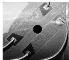
Monitoring of crack propagation during fatigue testing. The crack starts at an oil hole.
