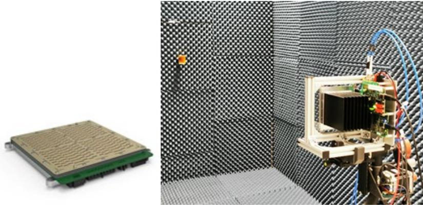
Fig 1. Testfixtures including Phased array antenna modules, Control interface modules, IF interface board, Mechanical stand, Cables and heatsink
