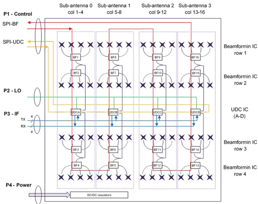
Fig 2. Functional diagram of the phased-array antenna module from Gapwaves
