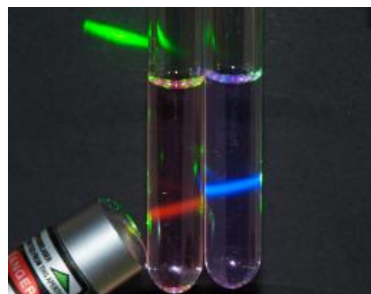
Figure 1. Example of normal Stokes emission (red) and upconverted anti-Stokes emission (blue) when irradiated by a green laser.
