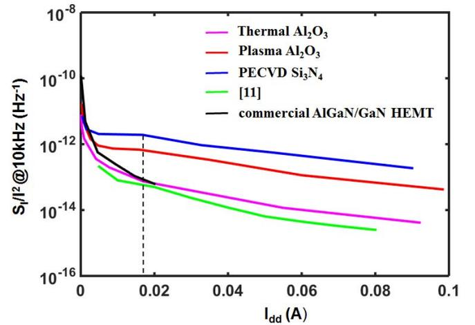
Fig. 2. Drain noise current spectra at 10 kHz versus the DC drain current of the three AlInN/AlN/GaN HEMTs at  $V_{dd} = 10$  V, a  $2 \times 50$   $\mu$ m commercial AlGaIn/GaN HEMT measured in [9] at  $V_{dd} = 10$  V and an AlGaIn/GaN device reported in [11] at  $V_{dd} = 5$  V. The dashed line indicates  $I_{dd} \approx 17$  mA.
