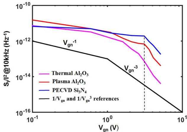
Fig. 3. Drain noise current spectra at 10 kHz of the three AlInN/AlN/GaN HEMTs versus the effective gate bias  $V_{gn}$  ( $V_{dd} = 10V$ ). The dashed line corresponds to  $I_{dd} \approx 17$  mA.
