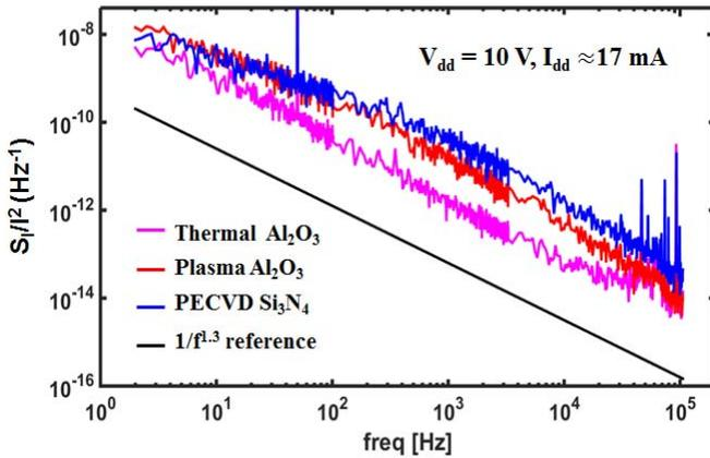
Fig. 1. Drain noise current spectra of the three AlInN/AlN/GaN HEMTs versus frequency at  $V_{dd} = 10$  V,  $I_{dd} \approx 17$  mA.
