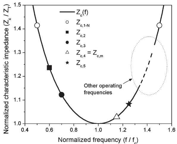
**Figure 4** Behavior of  $Z_c$  from (4) and values of  $Z_{c,i}$  for a multi-band quarter-wave transmission line case. For this example  $f_1 = 0.5$  GHz,  $f_2 = 0.6$  GHz,  $f_3 = 0.7$  GHz,  $f_4 = 1.15$  GHz,  $f_5 = 1.25$  GHz, and  $f_N = 1.5$  GHz are assumed. Other arbitrary operating frequencies are supposed in the range 1.35–1.45 GHz as well.
