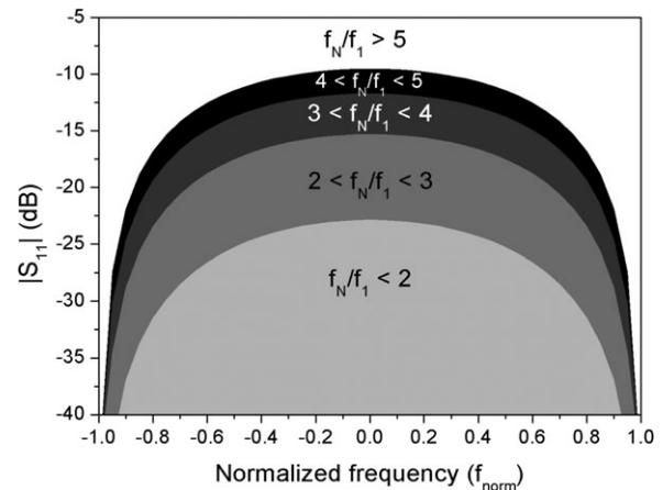
**Figure 6** Matching limitation for multiband quarter-wave transmission lines versus normalized frequency  $f_{\text{norm}}$  as defined in (16).
