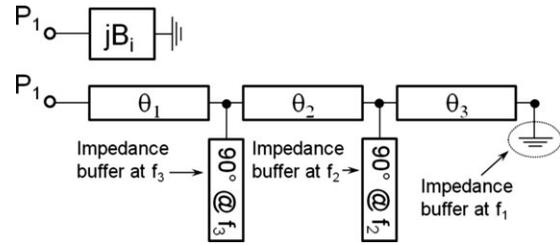
**Figure 3** Ladder network obtained applying the Impedance Buffer Methodology to synthesize the  $B_i$  susceptances for a triple-band quarter-wave transmission line.
