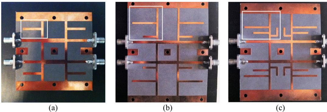
**Figure 9** Photos of the realized (a) dual-band, (b) triple-band, and (c) quad-band branch line couplers, whose sizes are  $65 \times 51$  mm<sup>2</sup>,  $75 \times 82$  mm<sup>2</sup> and  $73 \times 70$  mm<sup>2</sup>, respectively. The network based on the Impedance Buffer Methodology that synthesizes the desired values of  $B_i$  is highlighted in each figure by means of a white frame.
