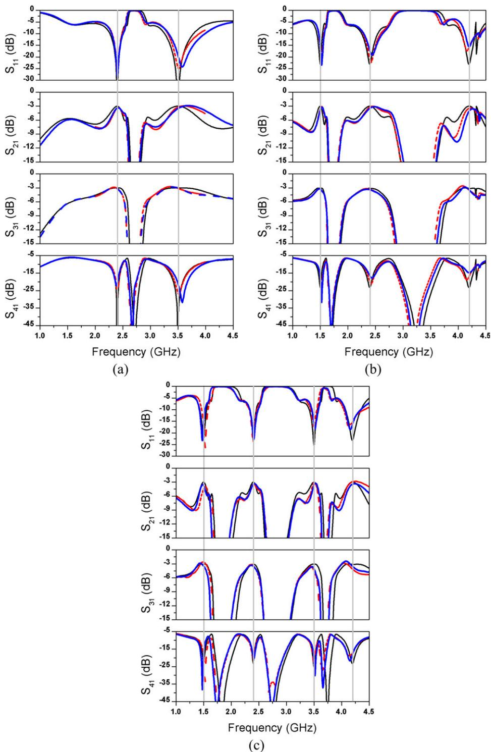
**Figure 10** Measured and simulated results of the (a) dual-band, (b) triple-band, and (c) quad-band branch line couplers.
