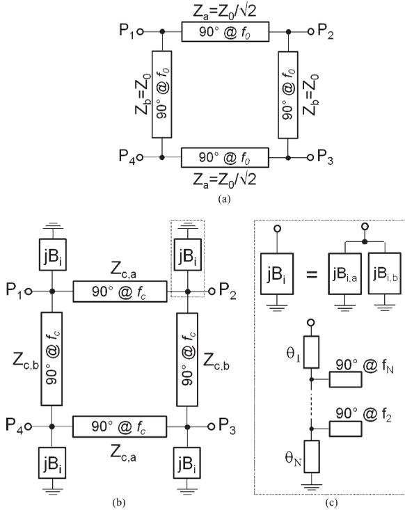
**Figure 7** Topology of (a) single-band branch-line coupler, (b) multiband branch-line coupler, and (c) multi-band network for the synthesis of the  $B_i$  susceptances.
