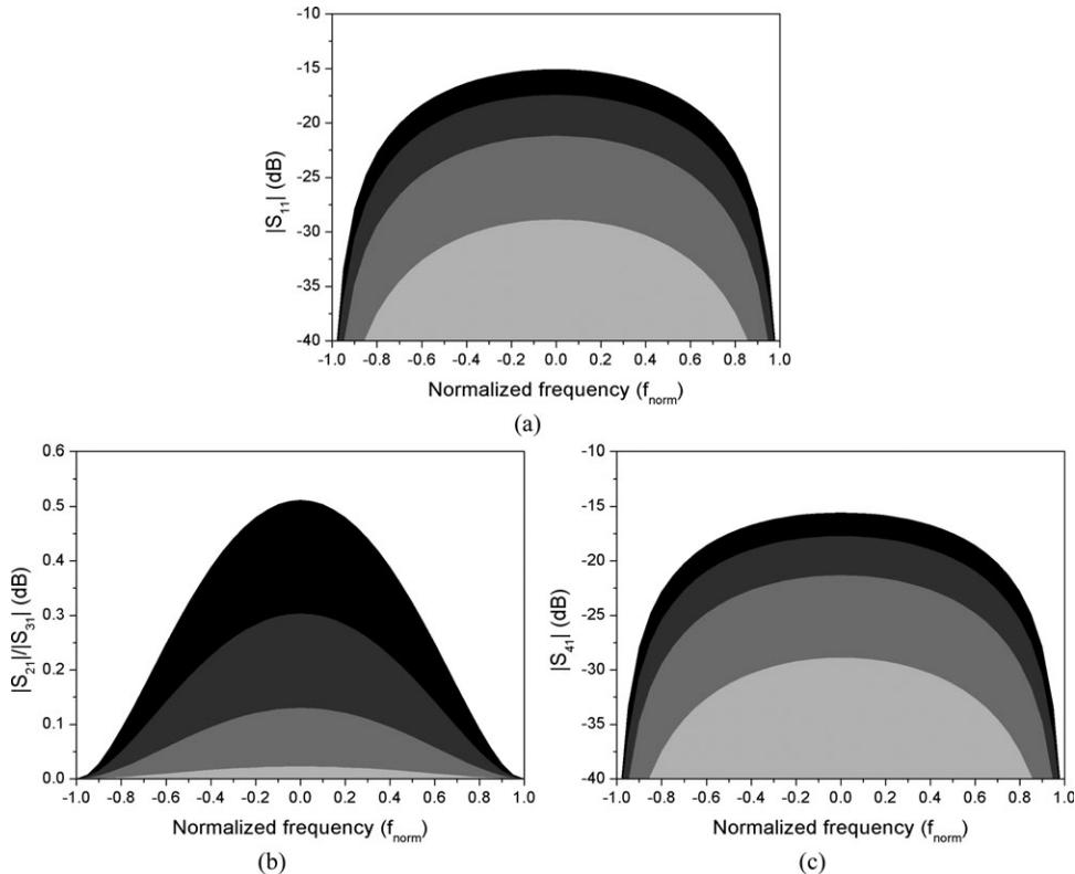
**Figure 8** Matching (a), balancing (b) and isolation (c) limitations for multiband branch-line couplers versus normalized frequency  $f_{norm}$  as defined in (16).
