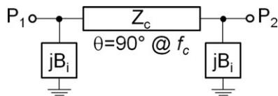
**Figure 1** Pi-shaped network which is equivalent to a quarter-wave transmission line at two frequencies.  $B_i$ ,  $i = 1,2$ , represent the susceptances at the two frequencies.
