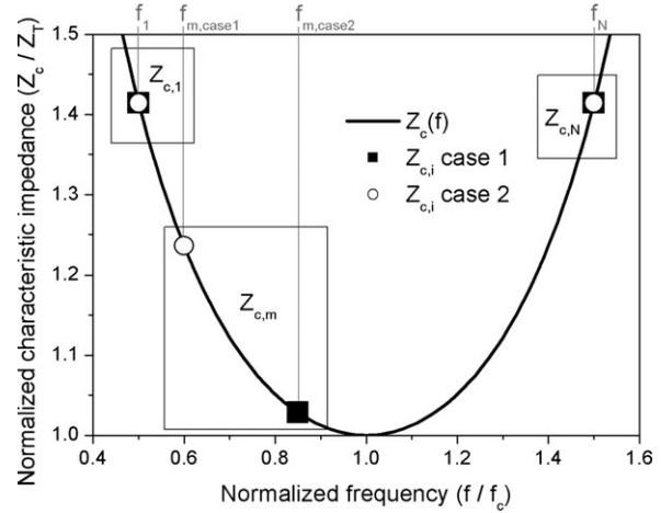
**Figure 5** Behavior of  $Z_c$  from (4) and two cases of  $Z_{c,i}$  having different matching limitations. For both cases  $f_1 = 0.5$  GHz and  $f_N = 1.5$  GHz are assumed, resulting in the same  $f_c$ ,  $Z_{c,1}$ , and  $Z_{c,N}$  values.  $f_m = 0.6$  GHz and  $f_m = 0.85$  GHz are assumed for Case-I and Case-II, respectively.
