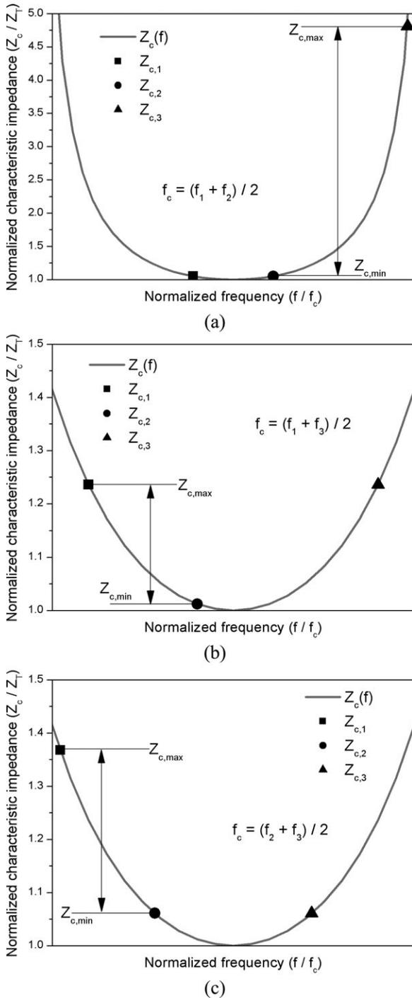
**Figure 2** Behavior of  $Z_c$  from (4) and values of  $Z_{c,i}$  for a triple-band quarter-wave transmission line case by assuming  $f_c$  as defined in (a) equation (12a), (b) equation (12b), and (c) equation (12c). For this example  $f_1 = 0.6$  GHz,  $f_2 = 0.9$  GHz, and  $f_3 = 1.4$  GHz are assumed.
