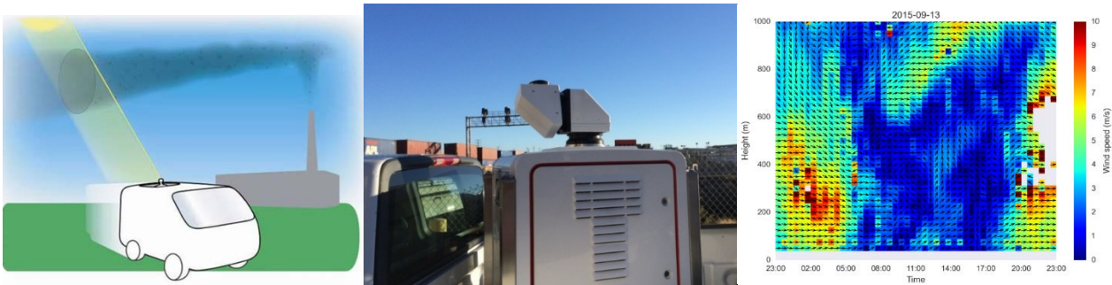
Figure 1. Left: The Chalmers solar occultation flux method which today is a European standard how to measure diffuse gas leakages of volatile hydrocarbons. Middle and right: a commercial stationary wind LIDAR (Light Detection and Ranging) measuring the 3D wind.
