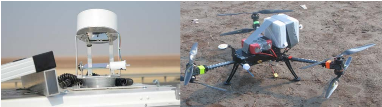
Figure 1. Left: The Chalmers IGPS solar occultation flux method which today is a European standard how to measure diffuse gas leakages of volatile hydrocarbons. Right: The Chalmers drone used to carry various sensors that will be applied in this project.
