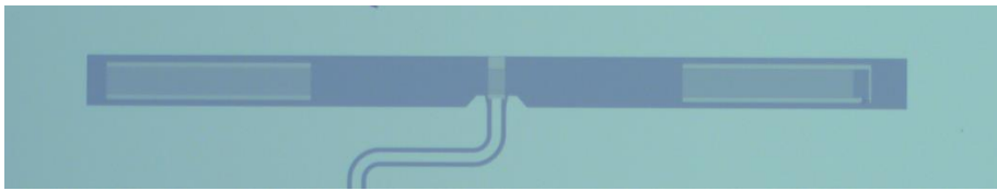
Figure 1: Surface acoustic wave resonator for quantum information. The centered interdigital transducer and Bragg reflectors are fabricated from Aluminium on a piezoelectric Gallium Arsenide substrate. The right-hand side reflector has an integrated Superconducting Quantum Interference Device (SQUID) to provide nonlinear coupling between the resonator modes.
