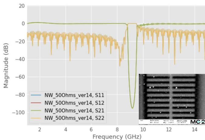
Figure 2 Simulation of the scattering parameters of a microstrip TWPA centered around the band gap. Insert: SEM image of a portion of non-linear microstrip line made at Chalmers.
