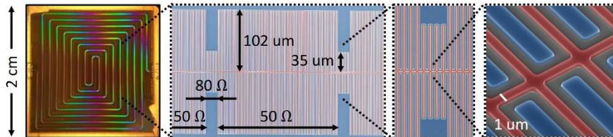
Figure 1 NbTiN TWPA developed by Malnou *et al.*
