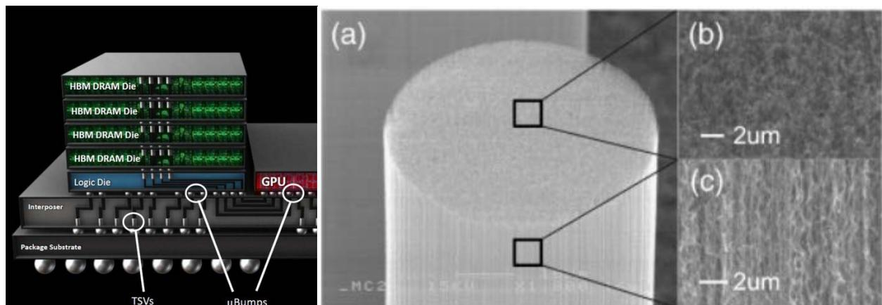
Figure: Left – A schematic of TSV implementation in modern 3D stacked IC devices. Right – A carbon nanotube bundle grown using the CVD process.
