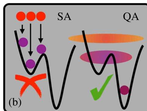
Fig1: A quantum annealer can find the minimum energy configuration of an energy landscape associated to the Hamiltonian encoding combinatorial optimization problems by exploiting quantum tunneling. From *Phys. Rev X* 5, 031026 (2015)
