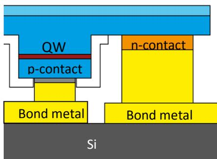
An UV-emitting thin-film flip-chip LED
