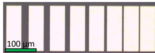
Fabricated TLM-pattern which is used to measure contact resistance to e.g. AlGaN
