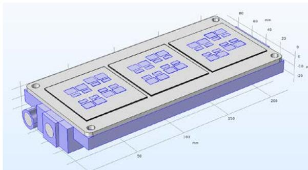
Figure 1. Schematic of the high-power IGBT module and heat sink with water cooling system.
