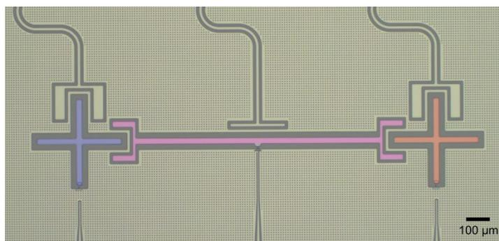
A system of two superconducting qubits (red, blue) can act as a heat engine. Micrograph courtesy of A. Bengtsson.
