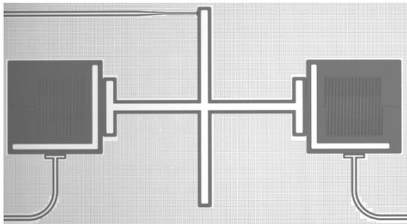
*Optical micrograph of a cross-shaped, flux-tunable coupling element between two lumped-element microwave resonators. (Design by S. Scharmer, unpublished)*
