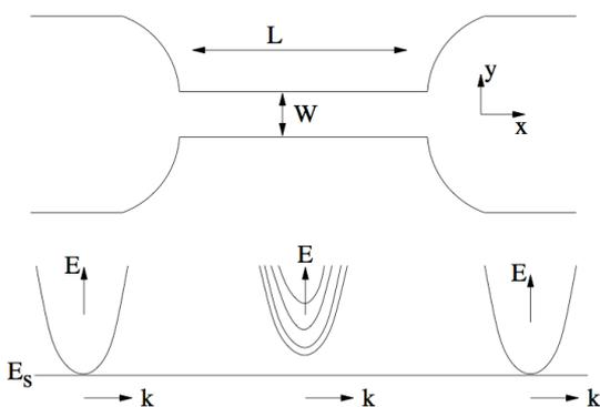
Fig. 2. Narrow conductor etched out of a wide conductor. In the wide regions the transverse modes are essentially continuous, but in the narrow region the modes are well-separated in energy.
