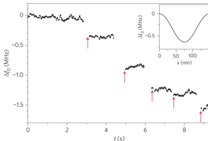
Figure 3: Yoctogram mass sensing with a nanotube, from J. Chaste et al. [Nature Nanotech. 7, 301 (2012)]. The red arrows mark the event when a single molecule attaches to the nanotube.
