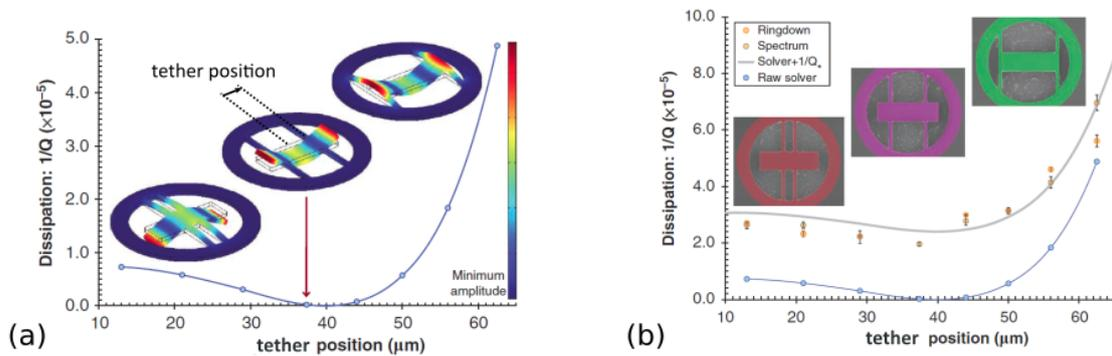
Figure 1: Mechanical dissipation in dependence of tether position, from G. D. Cole et al. [Nature Comm. 2, 231 (2011)]. (a) FEM simulation results, (b) comparison experiment and simulation results.
