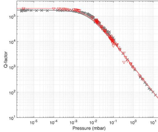
Figure 2: Mechanical quality factor in dependence of pressure, from A. Naesby et al. [Appl. Phys. Lett. 111, 201103 (2017)]
