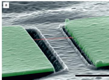
Figure 1: Suspended carbon nanotube. The scale bar is  $1 \mu\text{m}$ , from S. L. Bonis et al. [Nano Letters 18, 5324 (2018)]
