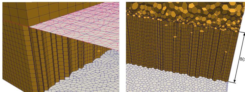
*Examples of unstructured grids for a wall-modelled LES of a turbulent boundary layer.*
