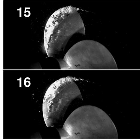
Figure 1: Two frames from a high-speed video of unsteady cavitation on a model-scale propeller in open water. Pereira et al.[2]
