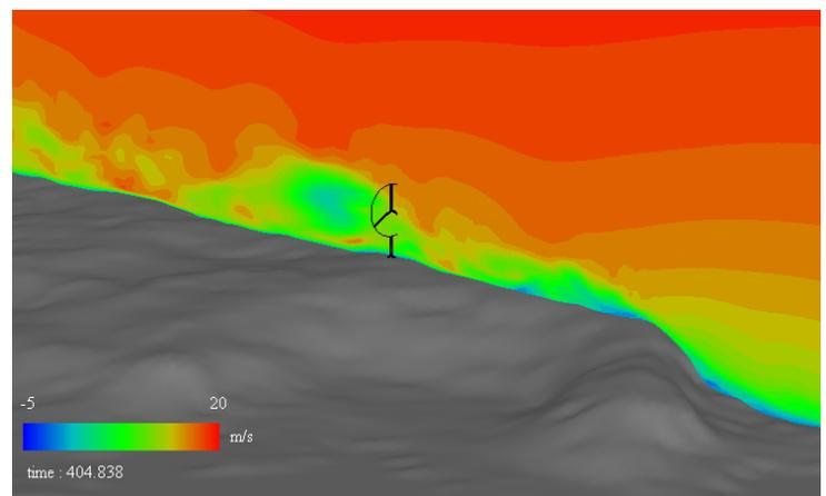
**Figure 1:** Schematic of the flow over complex terrains and CFD Simulation [6].
