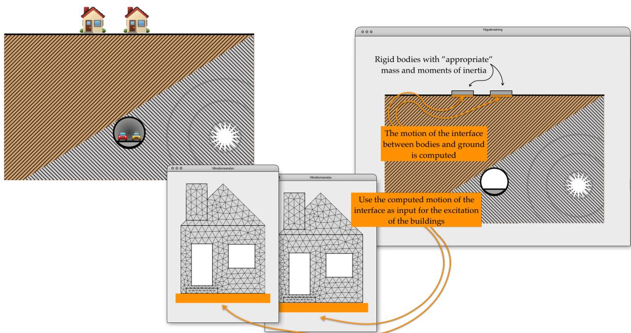
In addition to the present suggested Master Thesis project, a proposed parallel Master Thesis project ("Effects on buildings from blast induced vibrations – West link project") is focussing on the mechanisms of structural damage to buildings, and it is expected that a mutually beneficial flow of ideas, suggestions, and data between that project and the present one is possible.
