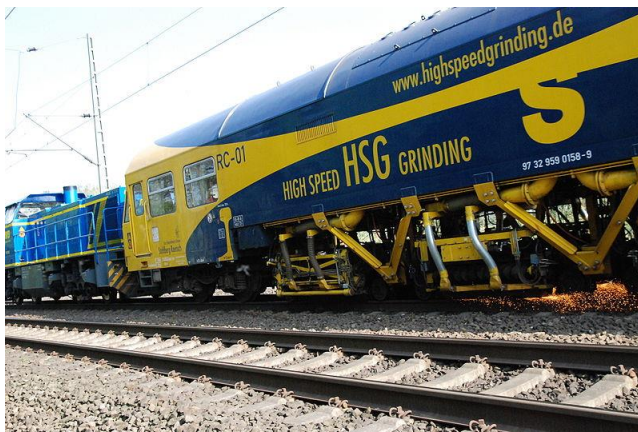
Figure 1: Highspeed rail grinding (left, CC-SA 3.0). Principle of rail milling (right, PD).
