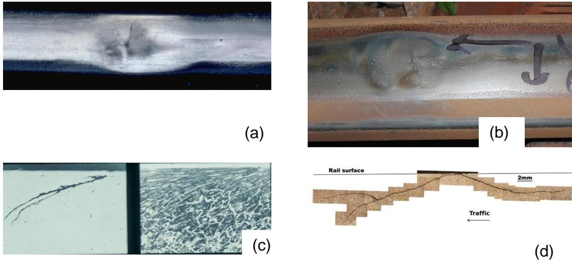
**Figure 1 Squat on left (from above and cross-section); stud on right (from above and cross-section)**
