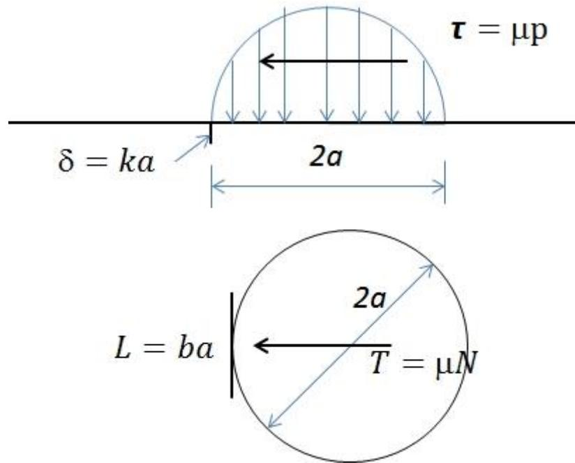
**Figure 2 Basic model to examine development of a stud from an initial vertical crack on the edge of the contact**
