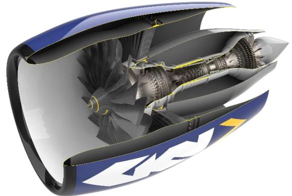
Figure 1 - Notional Type Design for Future Aircraft Engines
